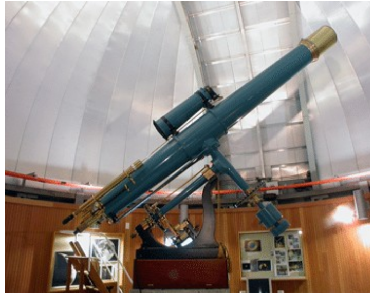
Figure 4: The 8 inch Clark refractor, an object in which art and science merge.
