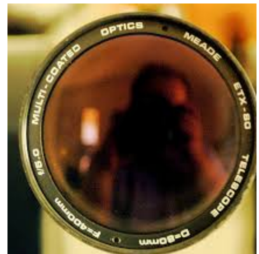
The aperture of a lens or mirror is the diameter of its light collecting region. The light-collecting ability of an objective lens or mirror is related to the square of the aperture.
